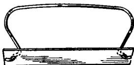
FIG. 10. A burnisher for inside of the lever horns.
