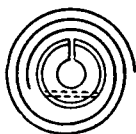
FIG. 54. The first coil of the spring should be at a distance from the collet equal to the distance between coils as shown here.
