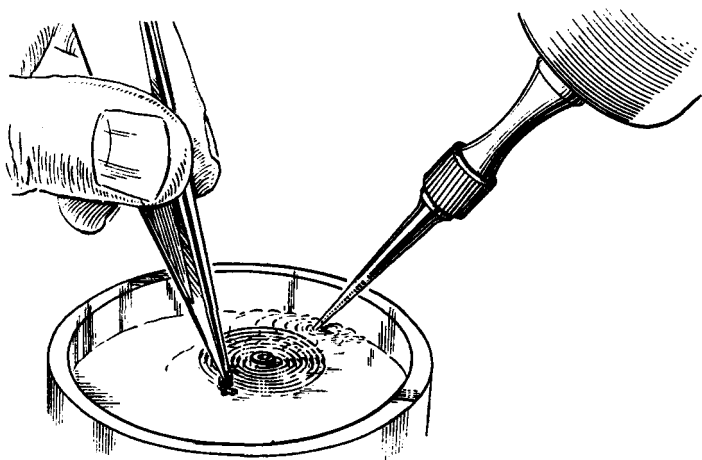
FIG. 14. Cleaning a balance spring in benzine by agitating the liquid with a bellows.
